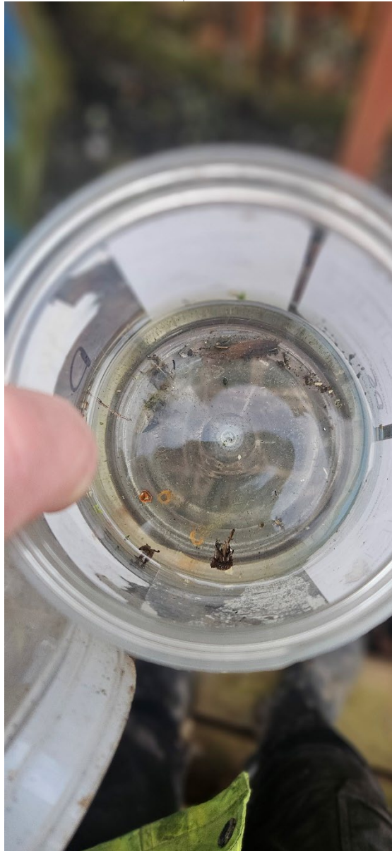
Photo 18: Example of large debris and organic material particles and even evidence of rust in D4
