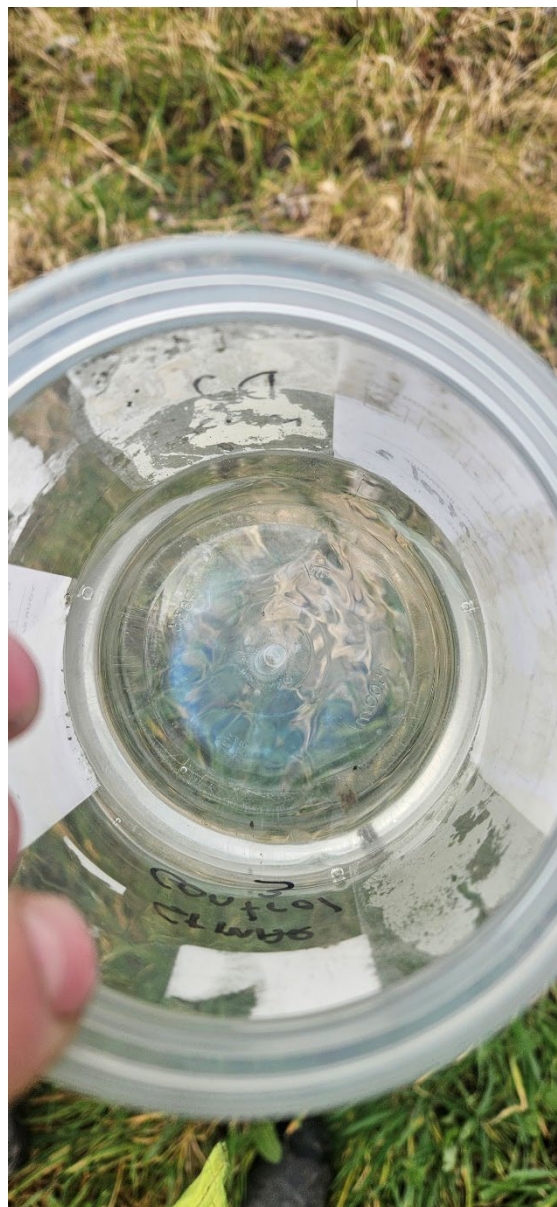
Photo 16: examples of the dust jar after mitigation measures (no debris and very little organic material) Control jar is placed approx. 50m from netting and treeline at hammermill side.
