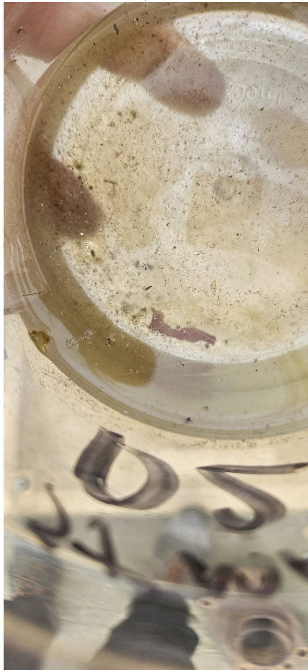
Photo 17: Example of large debris particles and even piece of metal at D2
