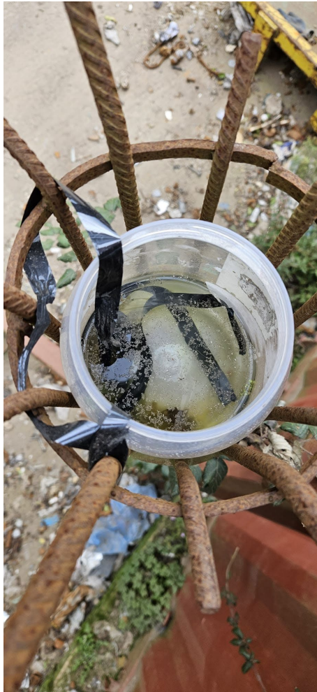
Photo 15: Another example of material fallen (tape and organic material) into a dust jar at D4
