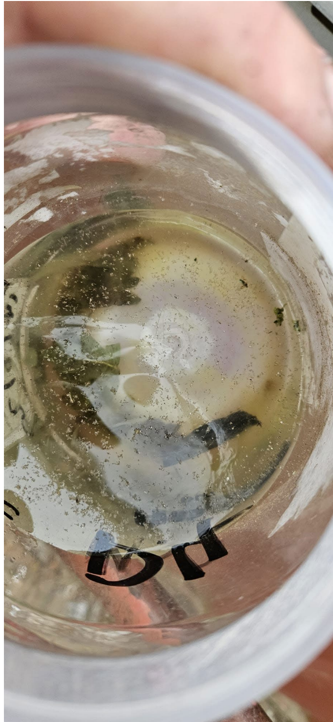
Photo 14: example of organic matter falling in dust jar at location D4 (only large leaves are removed before analyses)
