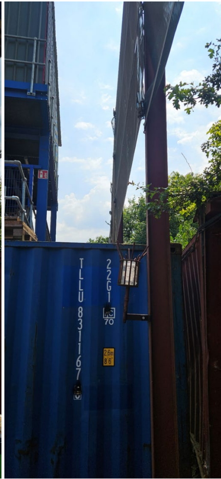
Photo 11 and 12 Dust location D5, container with higher flat surface directly next to collection point. Netting directly above collection point and at very close proximity the plant which is much higher than the collection jar. Allowing for debris to fall down into the jar
