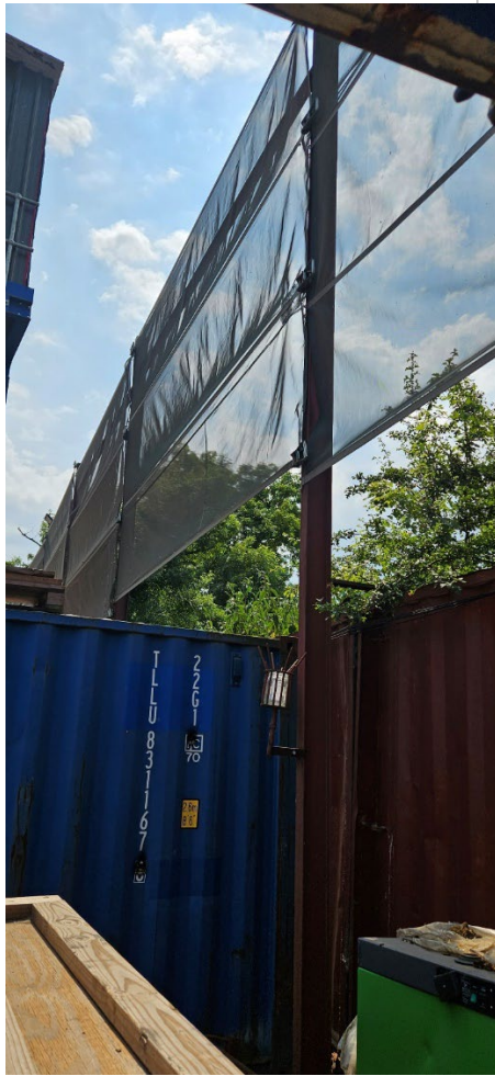
Photo 11 and 12 Dust location D5, container with higher flat surface directly next to collection point. Netting directly above collection point and at very close proximity the plant which is much higher than the collection jar. Allowing for debris to fall down into the jar
